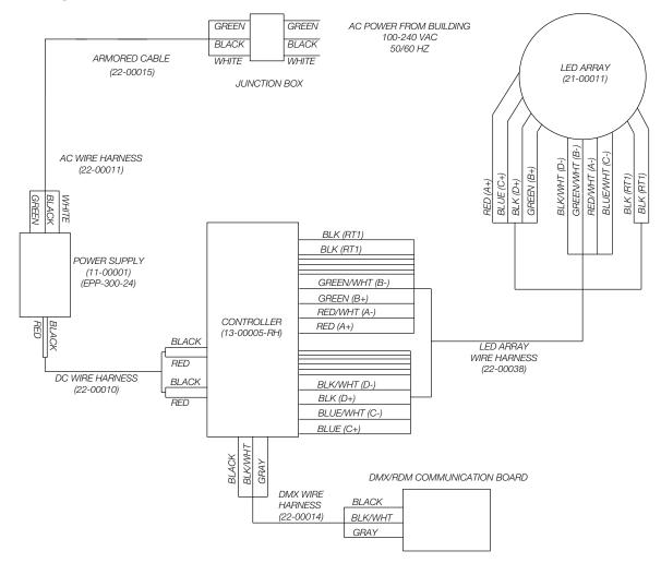
See Page 6 for instructions on how to secure the fixtures DMX/RDM Communication Connection.
